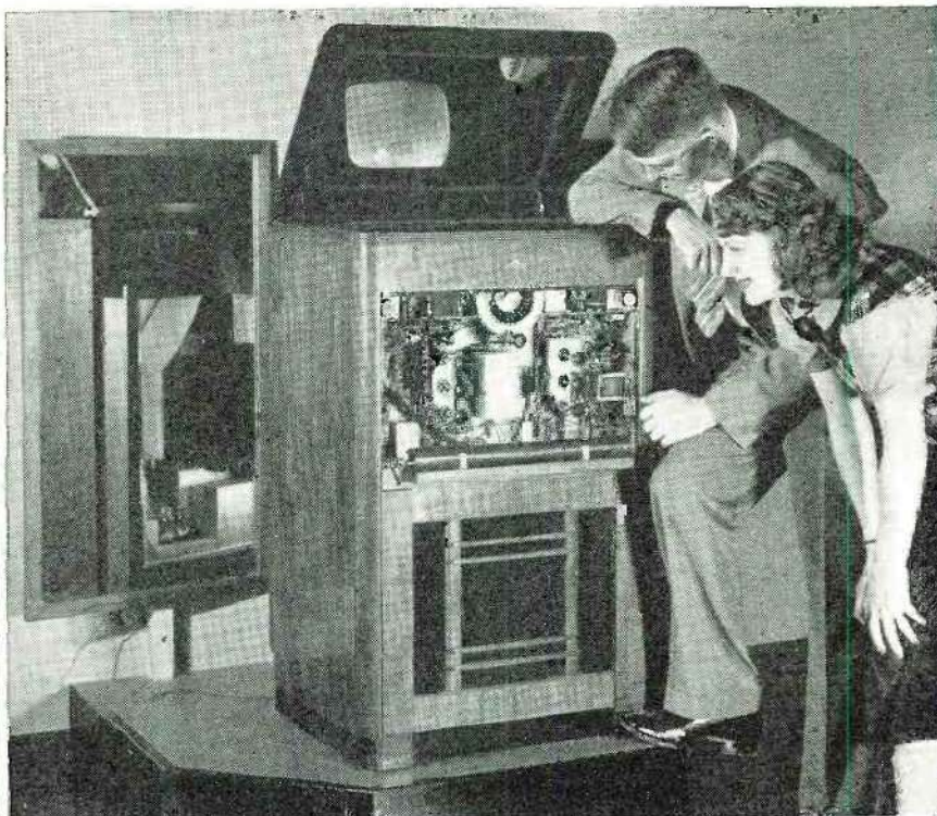
A television receiver for use by home groups. It uses 9" C.R. tube.
