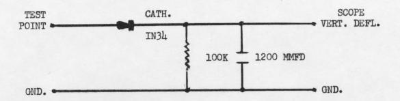
This circuit can only be used when the test point has no or very little d-c voltage on it.
