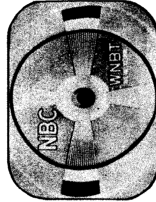
FIG. 19: HOR. LINEARITY MISADJUSTED - BUNCHES TO CENTER
