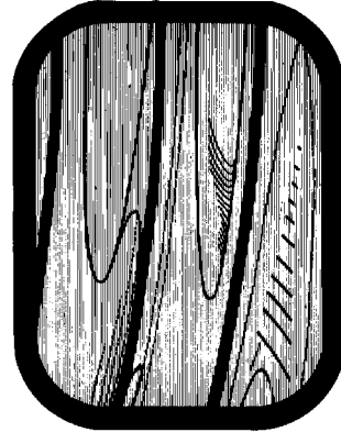
FIG. 41: IGNITION INTERFERENCE - HEAVY
