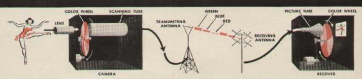
CBS EQUIPMENT employs wheel which rotates behind camera lens and separates the three basic colors of the image. Wheel's red, green and blue segments filter the light from subject so the colors pass through in succession. As in all TV, scanning tube changes lens image into electric signals which are broadcast. In
