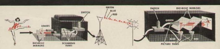
RCA EQUIPMENT directs red, green and blue light from the subject into separate lenses by means of a series of "dichroie" mirrors, each of which reflects only one color into the lens of the camera. Individual scanning tubes then translate the three lens images into broadcast signals. An electronic switching device allows
