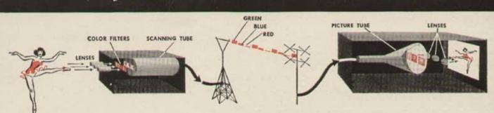
CTI EQUIPMENT has three camera lenses focused on the subject. Behind the lenses are mounted three color filters which produce red, green and blue images side by side on a single scanning tube. This triple image is transmitted over the air as a single picture. In CTI receiver this three-in-one composite image is re-
