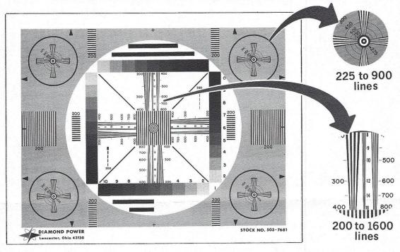
Diamond's advanced technology in the manufacture of High Resolution Closed Circuit Television Systems required an advanced quality test pattern to measure the increased picture quality.
