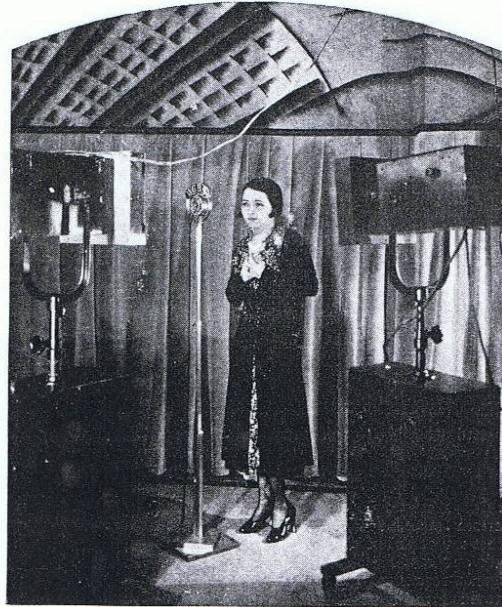
This is another scene taken in the interior of the Jenkins studio in New York, showing the WGBS "mike" picking up the voice, and, at right and left, the banks of photo cells for image pick-up
