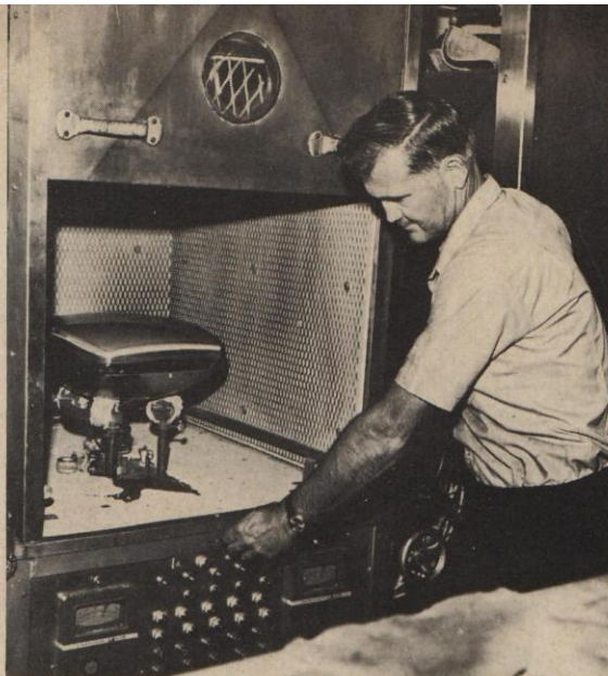
A tube is placed in the Windsor oven for baking. The temperature will be brought up to 240°F and evacuate the tube. This cycle normally takes two and one-half hours for a color tube.
