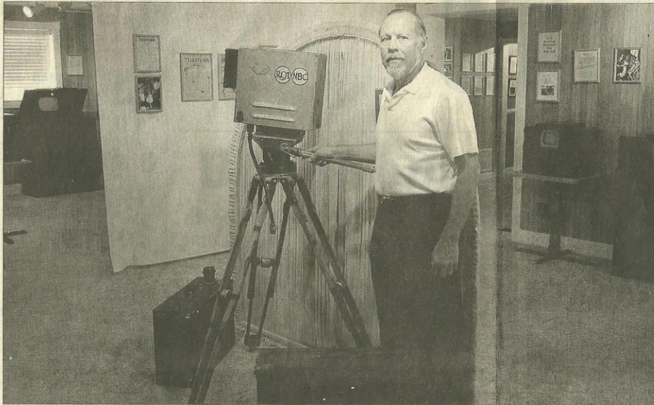
Steve McVoy poses with one of the two remaining RCA 1939 Iconoscope Cameras. This second generation remote camera was the first that could be transported by one car. The original cameras took two trucks to move.
