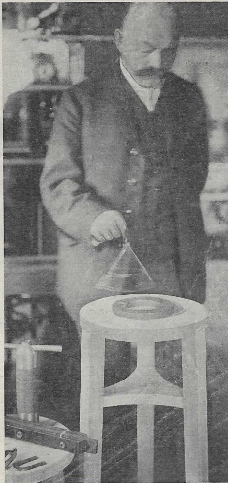
THE BRASS PENDULUM ACTUATED BY A RING MAGNET BELOW ILLUSTRATES THE PRINCIPLE OF THE OLD DIVINING ROD. WHEN WATER OR IRON WAS BELOW, AT NOT TOO GREAT A DEPTH, THE INSTRUMENT IN THE HAND MOVED
