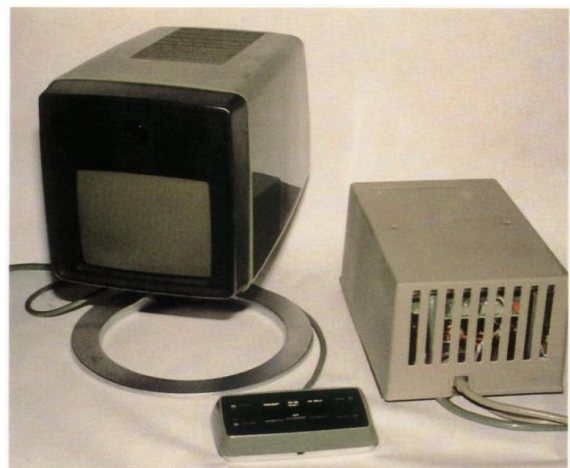
THE ORIGINAL PICTUREPHONE, MADE BY WESTERN ELECTRIC IN THE EARLY 1970S CONSISTING OF 1A DISPLAY UNIT, THE 72A CONTROL UNIT, AND 1A SERVICE UNIT.
