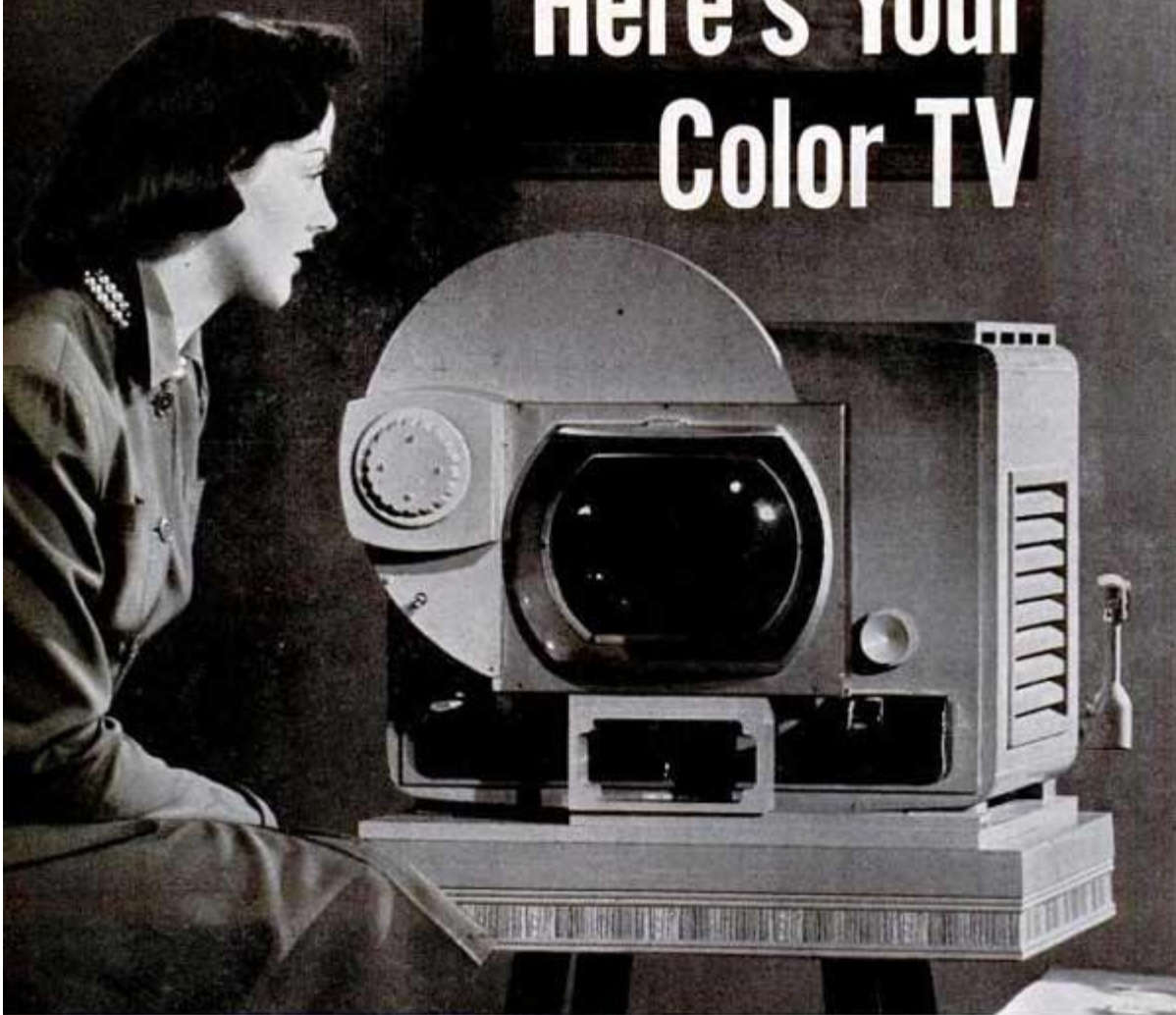
To convert this Zenith to color, CBS engineers added adapter in back, filter disk in front.
