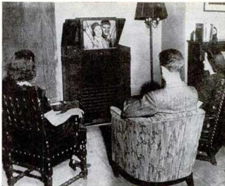
Clear, large-screen reception is a "must." In this RCA developmental job, the kinescope image is projected onto a mirror that reflects it onto the back of the translucent 13½ by 18-inch screen. The screen is retractable
