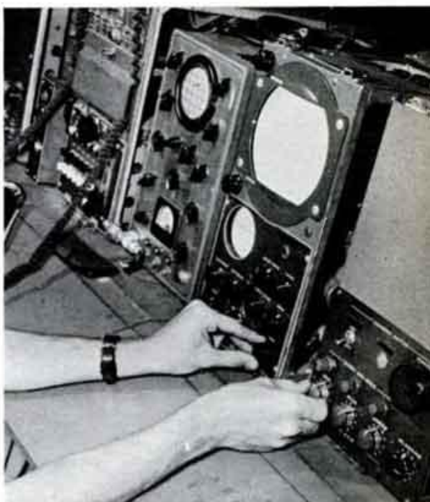
THE CONTROLS An extra panel (extreme right in photo above) adjusts the color-wheel motor and color balance in each camera. The technician's hand is on the knob that sets the amount of red in the picture. Adjacent knobs control blue, green.
