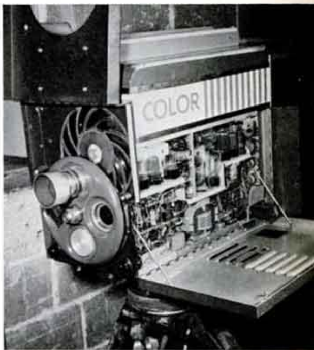
THE CAMERA Only when covers are opened can alterations that convert camera to color be seen. Twelve-segment filter disk (above lens turret) spins on long shaft running through camera to motor in rear. Viewfinder shows black-and-white picture.
