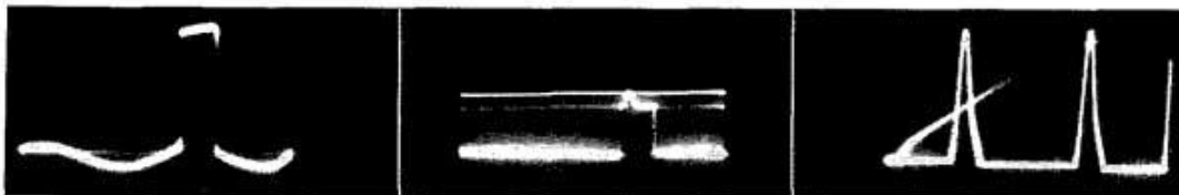
Fig. 2 (left) — Oscillogram of the vertical oscillator impulse. Fig. 3 (center) — Oscillogram of the vertical blanking and sync pulse. Fig. 4 (right) — Horizontal oscillator impulse oscillogram.
