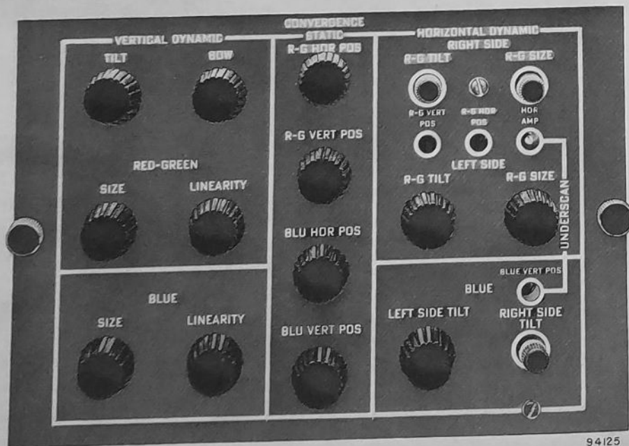
Figure 12. Control Side, Convergence Chassis
