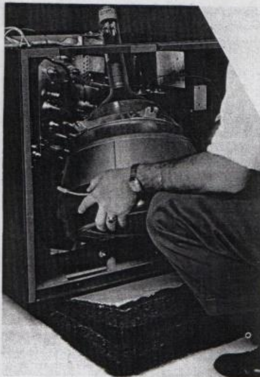
Fig. 75—Placing Kinescope in Cabinet
