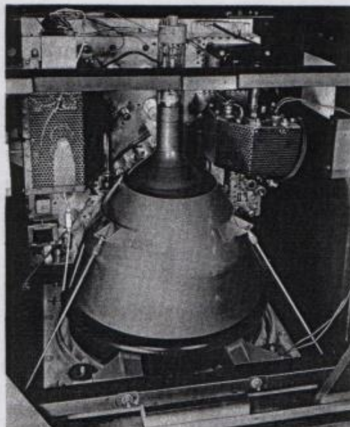
Fig. 76—Kinescope Mounted in Cabinet
