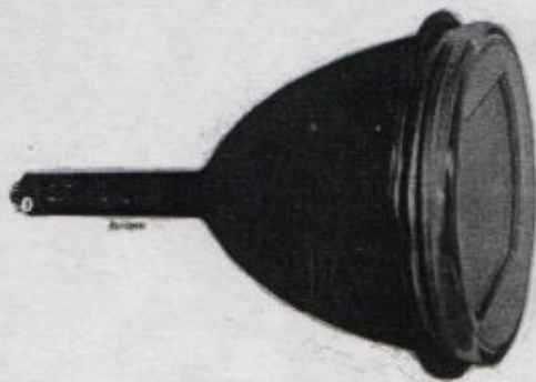
Fig. 10—RCA 15GP22 Tricolor Kinescope
