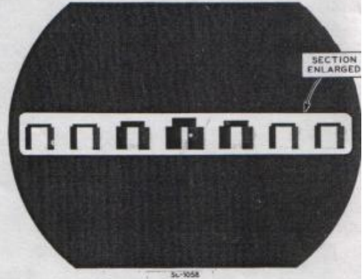
Fig. 95—Horizontal Convergence Amplitude Incorrect
