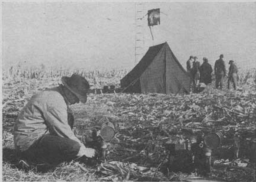
Fig. 4. Gasoline generator used to energize microwave field testing equipment in connection with preliminary work on the $500,000 microwave relay from Chicago to Milwaukee.
