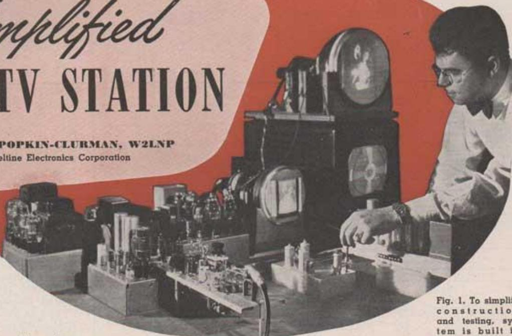
Fig. 1. To simplify construction and testing, system is built in separate units.
