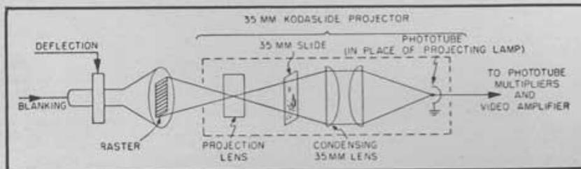
Fig. 3. Method for using cathode-ray tube as light source for 35mm transparencies.
