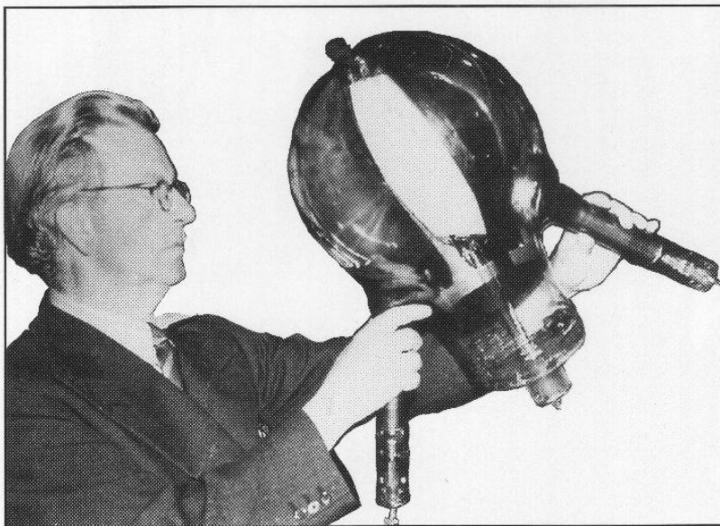
J.L. Baird with his Telechrome, the world's first multi-gun colour television tube. August 1944.
