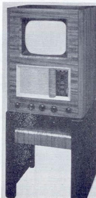
Below: The Burndept console television receiver. Picture size 10 ins. by 8 ins.
