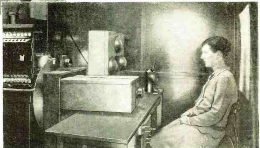
Fig. A at the left and Fig. B below show the relative positions of the apparatus used in transmitting by radio the image of the girl. In Fig. A the arc lamp is at the left and, between the revolving disc and the square frame holding the photoelectric cells, is the small square wooden holder carrying the lens. The amplifier is in the two boxes at the right. The grouping of the photoelectric cells is shown in Fig. B below, three being visible and a fourth behind the amplifier boxes. Note the microphone at the right and the lines of light and shadow on the girl's face in Fig. B; and the enlargement in Fig. C, at the lower left.
