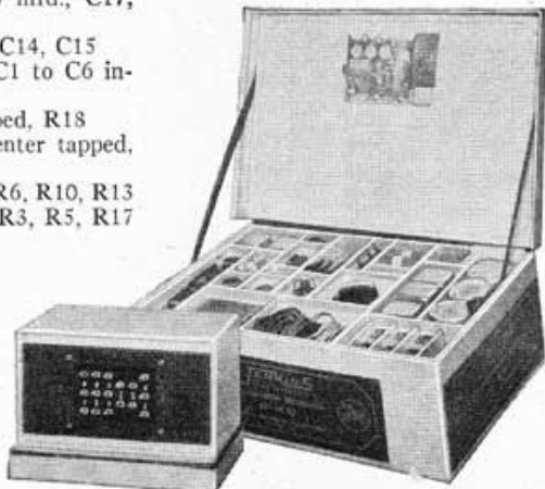
The television receiver kit, showing power transformer at left. All necessary parts are included and numbered. Complete instruction book and diagrams are included in the kit
