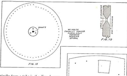
tically form a tube in the disc of some length. Thus if the light approaches the disc at an angle only slightly off of the perpendicular, much of it will be cut off. In looking through a gun barrel or mailing tube we must allow the light to come straight to our eyes. However, light from a picture must come from various directions because of the size of its area and hence the holes in the disc must be beyeled.
