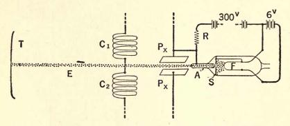
Fig. 3.—Schematic layout of the necessary components of a cathode ray tube used to make visible oscillating currents. The electron stream created by the hot filament F is forced out of its normal path by charges on the plates  $P_{\rm X}$  and by currents in the coils  $C_{\rm r}$  and  $C_{\rm 2}$ . The electron stream produces a visible effect on the screen T. This principle has been applied to the reproduction of television pictures.
