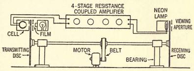
Fig. 73.—Diagram showing the simple arrangement of apparatus for a television transmitter and receiver which any experimenter may set up at home. Perfect synchronism is brought about by the simple expedient of mounting the transmitting and receiving scanning discs on the same shaft.
