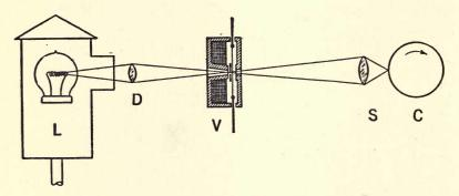
Fig. 13.—Principal parts of the Bell picture receiver. L is the light house, D a condensing lens, V the light valve, S a condensing lens and C the cylinder carrying the photo-sensitive paper. (Courtesy Bell Telephone Laboratories, Inc.)
