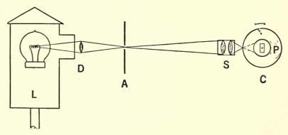
Fig. 11.—Simple elements of the Bell Telephone phototelegraphic system. L is the light house, D a condensing lens, A an aperture, S a projection lens, C the transparent cylinder, and P the photoelectric cell. (Courtesy Bell Telephone Laboratories, Inc.)
