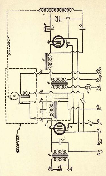
is connected to the output of a standard broadcast receiver. This is really the printing apparatus which is Fig. 10.—More conventional diagram of the connections used in the Cooley Rayfoto receiver. This apparatus controlled by the signal received from a broadcast outfit. The high-voltage discharges appears at the point of the needle which is shown resting upon the cylinder.
