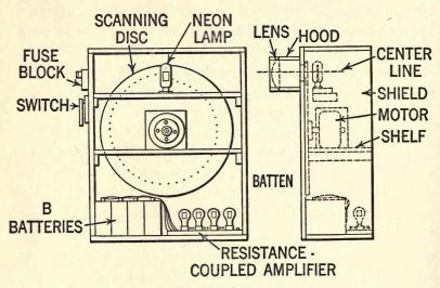
Fig. 78.—General arrangement of the parts making up a television receiver. The box is made of three-quarter-inch white pine painted black inside to prevent reflection and to sharpen the outline of the received picture.
