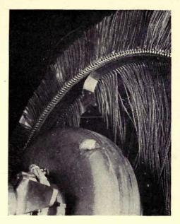
Here is a part of the 2500 separate wires running from the contacting device to the 2500 tinfoil electrodes on the large neon tube of the Bell Telephone television system. The revolving contactor connects each one of the electrodes once during each revolution. Naturally, this revolving arm runs in synchronism with the scanning device at the transmitter. (Photo Courtesy Bell Telephone Laboratories, Inc.)
