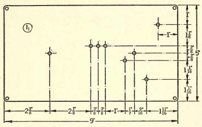
Fig. 74.—How the front panel of the short wave tuner is laid out to be drilled.
