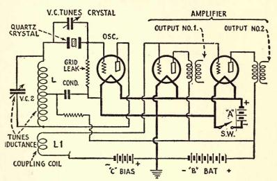
Fig. 67.—Method used in incorporating a quartz crystal in an oscillating circuit. When so placed, a crystal will actually control the frequency of oscillation. Due to this, such crystals have been successfully employed in bringing about synchronism between television receivers and transmitters. (Courtesy "Radio News.")
