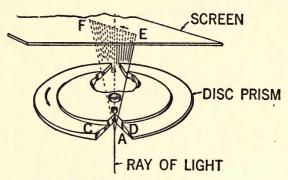
Fig. 59.—Revolving glass prism used for scanning in the Jenkins system of picture transmission. (Courtesy Q S T.)
