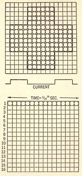
Fig. 56.—Graphic and simplified analysis of the scanning problem. This shows the number of picture units involved in the transmission of a black cross using a scanning disc with only 16 holes.
