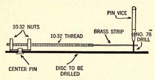
Fig. 64.—Drilling jig used in accurately locating and drilling the holes in scanning discs. This jig takes advantage of the fact that a 10-32 screw thread causes a rod to advance .015 of an inch for every half revolution.
