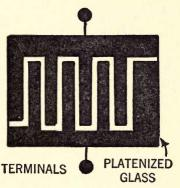
Fig. 52.—Wein selenium is constructed from a platenized piece of glass, the electrodes being formed by separation of the platinum surface into two parts. A thin film of selenium occupies the space between the two surfaces.
