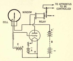
Fig. 18.—How a photoelectric cell is used to control a relay. When used in this manner, a cell will cause a beam of light to operate large machines like electric motors, horns or bells. If more stages of amplification are used, a less sensitive relay may be employed.
