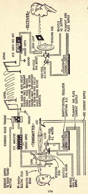
Fig. 68.—Showing how a quartz crystal oscillator is connected to a special high-frequency synchronous motor. Two (Courtesy Experimenter oscillators tuned to the same frequency are used, one at the transmitter and one at the receiver. Publishing Co.)
