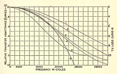
Fig. 31.—These curves illustrate in a graphic way the equivalent transfer admittance of various apertures. (Courtesy Bell Telephone Laboratories, Inc.)
