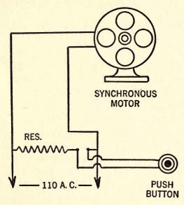
Fig. 65.—Showing the method of reducing momentarily the speed of a 6o-cycle synchronous motor by inserting a resistance with a push button.
