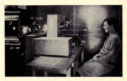
The arrangement of the scanning apparatus used at the General Electric Co., Schenectady. This is similar to the system sketched in Fig. 63. D is the light house of the arc lamp, G, the scanning disc, E the lens, F the photoelectric cell, and H the microphone. The dotted lines show the path of the scanning beam which is reflected from the face of the performer to the three sensitive photoelectric cells.
