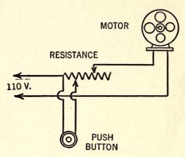
Fig. 66.—One method used to control the speed of a fractional horsepower motor with a small resistance and a push button which is constantly held in the hand of the operator. Two contacts are arranged on the resistance to enable the operator to obtain close adjustment.
