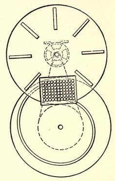
Fig. 58.—Scanning system first employed by the English television experimenter, Baird. As will be seen, Baird used a continuous spiral, the light being moulded into round beams by means of a cellular structure made up of round metal tubes.
