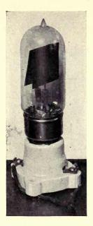
A special neon lamp with electrodes measuring 1½ x 1½. Such lamps are connected in the output circuits of television receivers.
