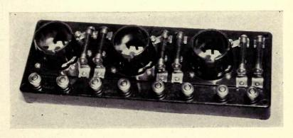
An ordinary resistance-coupled amplifier that may be employed for the amplification of picture signals. Such amplifiers are better adapted to this use than are amplifiers employing transformers as inter-stage couplers.
