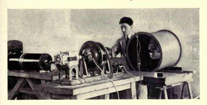
The electrical apparatus involved in the Belin-Holweck television transmitter. The photoelectric cell is mounted at the focal point of a large concave mirror which in turn is mounted at the end of the large cylinder shown. A cathode ray receiver is used in this system.
