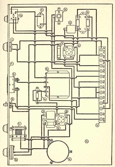
Fig. 9.—Layout and connection necessary for a receiver of the Cooley type. At A there is shown the "corona coil" which generates the high-voltage used in exposing the photo-sensitive paper wound upon the receiving cylinder.
