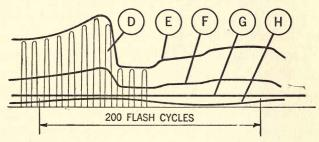
Fig. 72.—D. Neon lamp flashes, 40,000 per second. E. Flash energy applied to delineate picture on screen. F. Energy reflected by the small fixed mirror, Fig. 1, to fall upon the chopper. G. Maximum illumination required on the photoelectric cell to compensate for one per cent slow speed. H. Approximate synchronizing cycle made up of 200 flashes.
