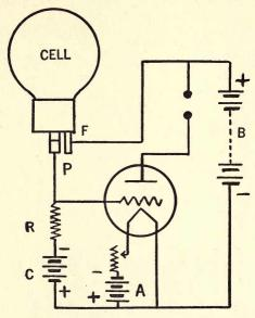
Fig. 17.—Connections for a single tube photoelectric cell amplifier. The resistance R will be found to vary, ½ megohm being about correct for Burt sodium cells. Other type cells will probably require higher resistances. The output of this amplifier may be fed to another amplifying system.
