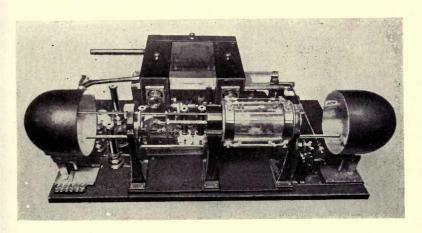
The transmitter of the Ranger system. As in all other photo-telegraphic systems, the picture is progressively explored with a fine pencil of light.
