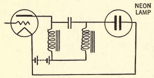
Fig. 45.—Use of two chokes and one set of B batteries in connecting a neon lamp to the output circuit of a television amplifier.
