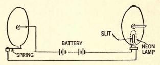
Fig. 69.—Simple indicator of synchronism. When the glow of the neon lamp is seen, this indicates that the wheel at the transmitter is running in perfect step with the wheel at the receiver.
