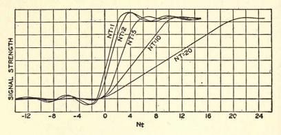
Fig. 29.—Distortion in an elementary frequency change as caused by a square aperture and ideal frequency restriction. (Courtesy Bell Telephone Laboratories, Inc.)
