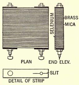
Fig. 49.—Townsend selenium shown here is made up of two separate sets of brass plates properly insulated from each other. The spaces between the plates are filled with molten selenium.
