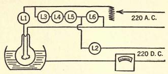
FIG. 25.—Another method of depositing sodium in the construction of photoelectric cells. The drawback of this system, as far as the amateur is concerned at least, is the necessity of having two sources of 220-volt current.
