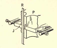
Fig. 12.—Details of the light valve used in the Bell phototelegraphic system. The ribbon R, which is arranged in the magnetic field of the magnet P, is moved slightly upon the passage of the picture current. This slight movement permits light to pass. (Courtesy Bell Telephone Laboratories, Inc.)
