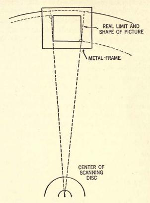
Fig. 77.—This diagram shows how the picture frame is cut to accommodate the size of the scanning disc used for reception.
