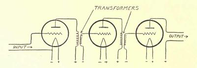
Fig. 22—Use of a series of three vacuum tubes (represented by circles) with transformers in a circuit to amplify television signals.
