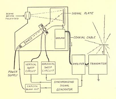
Fig. 31—Diagram of the units involved in a television transmission apparatus; the television camera (upper left) converts the light values into electric impulses which leave the signal plate of the camera cathode ray tube, pass through a first stage of amplification, and then (by means of coaxial cable) to the other amplifiers and the transmitting mechanism, located outside the television camera, and usually also some distance from the television studio.
