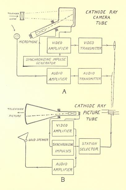
Fig. 7—Diagram of the various elements which are involved in a complete television system of the electronic type. A, transmitting apparatus; B, receiving apparatus.
