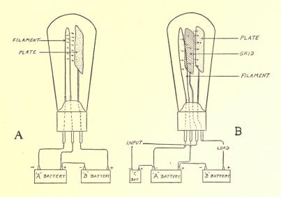
Fig. 19—A two-element vacuum tube: A, with only filament and plate; and a three-element vacuum tube: B, with a grid inserted between the filament and plate.
