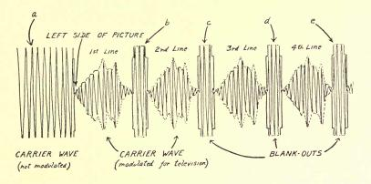
Fig. 35—Representation of the carrier wave and television signal modulation. At the left (a) is the unmodulated carrier wave, as it is during the absence of television signal modulation; during this time the vertical synchronizing impulses are applied. The modulation corresponding to four lines of the picture is indicated. Horizontal synchronizing impulses are applied at (b), (c), (d) and (e) while there is a pause between lines being transmitted.
