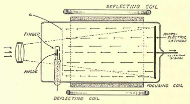
Fig. 39—Diagram of the Image-dissector type of camera tube. At (a) is the invisible electron image plane, formed by the electrons leaving the light-sensitive cathode at the right-hand end of the tube. The focusing and deflecting coils are outside of the tube.
