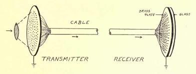
Fig. 4—Representation of the Carey system for simultaneous transmission of picture elements of a television image. 1880.
