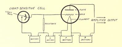
Fig. 20—A vacuum tube (represented by the larger circle) used as an amplifier of the light modulated current produced in a light-sensitive cell (represented by the smaller circle).
