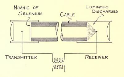
Fig. 5—Representation of the Morse system for simultaneous transmission of picture elements of a television image. 1893.
