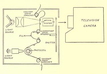
Fig. 40—Use of a film-scanner in converting motion picture scenes into television images. The motion picture projector is outlined in section view at the left.
