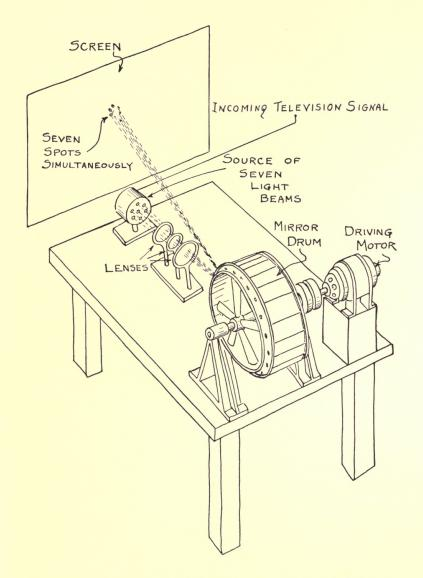
Fig. 11—The mechanical television system developed by Alexanderson, which used a mirror drum for scanning.
