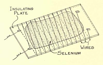
Fig. 2—Construction of an early type of selenium cell.
