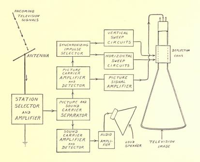
Fig. 53—Plan of a television receiver.
