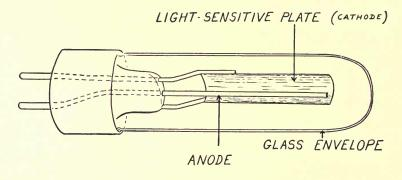
Fig. 3—Construction of a photoelectric cell.
