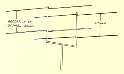
Fig. 49—A dipole television antenna, with a shield (looking like the receiving portion) to absorb unwanted signals.
