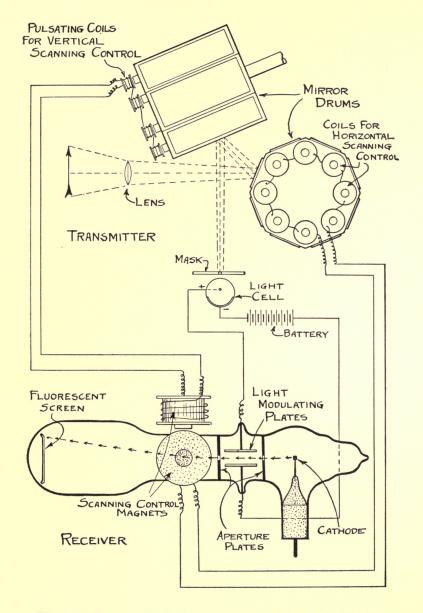
Fig. 17—An actual television system developed by Rosing, 1907, involving a mechanical scanning device in the transmitter and an electronic one in the receiver.
