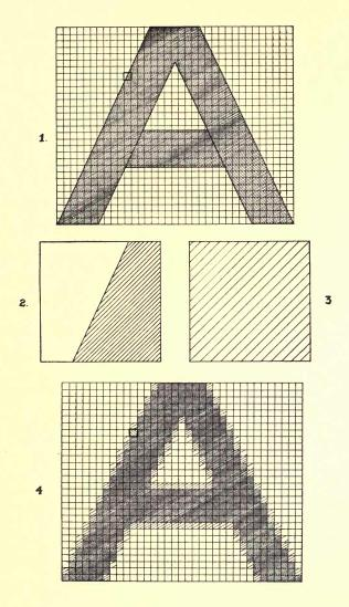
Fig. 6—The upper figure represents a letter "A" analyzed into 30 lines of 35 picture elements each. Some picture elements will be white, some black; but some—as in small square—will be partly white and black. An enlargement of this small square is shown at 2, while 3 shows the same square as it would appear on a television receiver. The complete letter "A" as it would appear on a television receiver is shown in 4.
