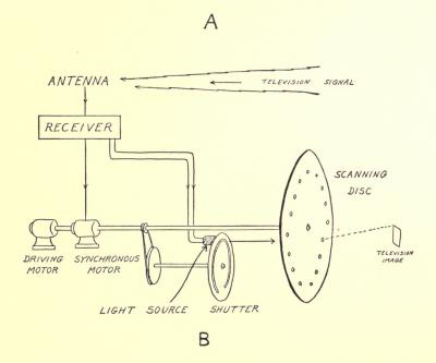
Fig. 9—An early Baird television apparatus.
