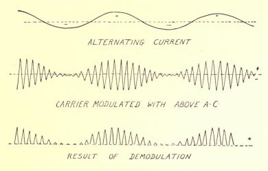
Fig. 24—Amplitude modulation of a carrier current.
