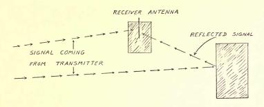
Fig. 48—Diagram showing double signal reception by an antenna; one signal coming direct from the transmitter, the other being reflected from a tall building behind the home of the televiewer.
