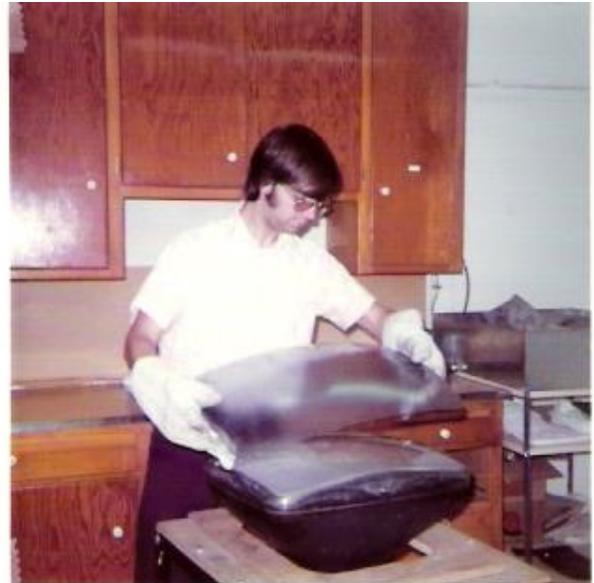
The oven photo shows the power lift. The added second support rod is just to the left of the tube neck. The 12v battery charger is on the floor to the left of the bombardier. The direction switch and car power window motor can be seen on a pad under the bombardier. A diagram of the power lift setup:
