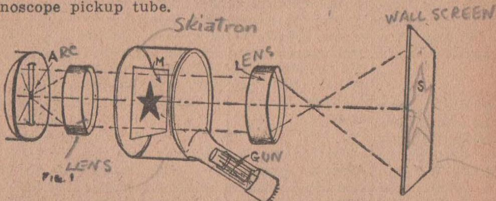
The coating on the plate may be a thin film of a single chemical salt or combination of salts such as certain alkaline iodides, bromides or chlorides, that have been found to discolor under electronic bombardment. The illumination may be from any source that has enough power to give the required brilliance.
