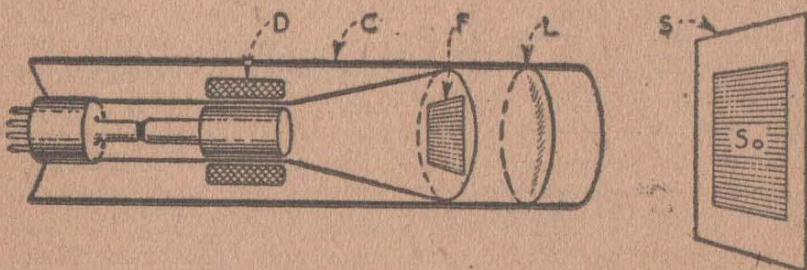
Problems that are inherent with the design of a projection tube are the same as those found with the ordinary tube, but the difficulties of their solution are much greater, viz., deterioration of the cathode emitter surface, burning of the fluorescent screen with high intensity electron bombardment, and the lowering of the vacuum by the degassing of metal parts by high speed bombardment.
