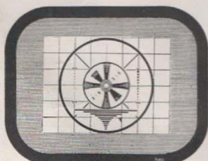
TOO SMALL HORIZONTALLY AND VERTICALLY —Adjust both HORZ. SIZE and VERT. SIZE controls on rear of set.
