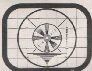
CORRECTLY ADJUSTED —Pattern is clear, steady. Proper contrast between black, white and various shades of gray.
