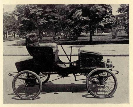
This horseless carriage is thought to be the first to have the engine under the hood in front.
