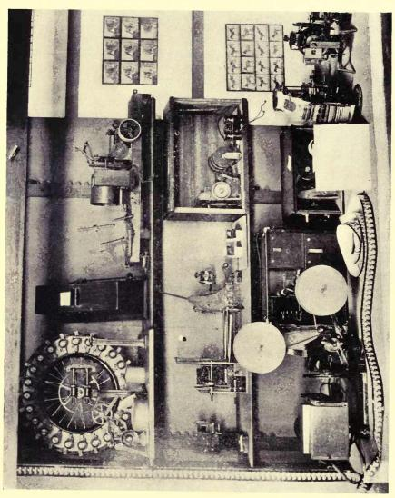
Mr. Jenkins early motion picture apparatus, film slitters, perforators, cameras, developers, printers, projectors, etc., on exhibit in U. S. National Museum since 1895.
