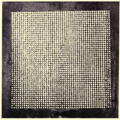
Face of the Jenkins Plate Receiver. It has 2,304 elementaryarea light-sources, arranged in 48 rows with 48 in each row. Persistence of light of each elementary area is substituted for persistence of vision, of the old spirally arranged disc-aperture method.
