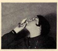
The card can't be blown off by blowing through the spool (if the corners of your mouth don't leak)
