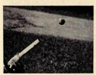
Showing how stream of air at 45° will hold ball suspended above ground
