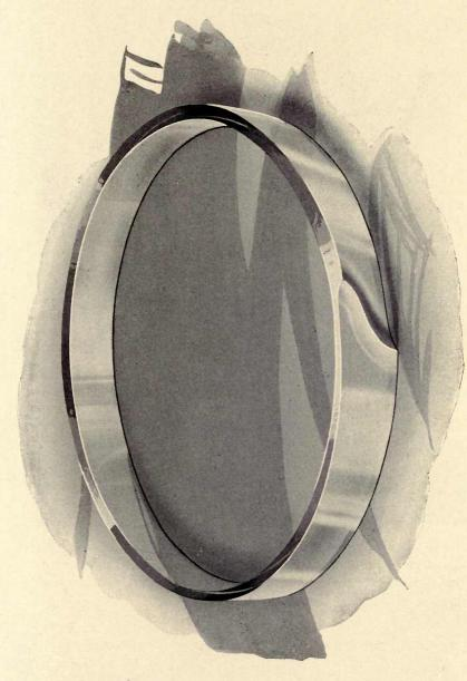
Prismatic ring (band ring type). In rotation, gives oscillation to a beam of light passing therethro.
