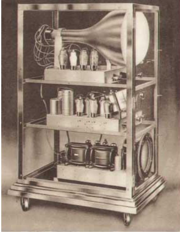
THE COSSOR THREE "DECK" TELEVISION CHASSIS —Above the upper deck is the Cossor Cathode Ray Tube. The middle section houses the radio receiver, while below is the power pack and moving-coil speaker.
