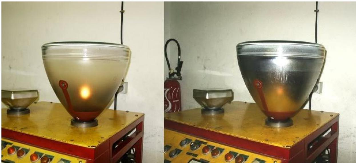
After the coating has been applied, the tube goes into the oven at 410°C to bake out the remaining lacquer. There is now a thin coating of phosphor and aluminum on the bulb face, separated by the space formerly taken up by the lacquer. A picture tube layer cake! After baking out the lacquer, blow out the fumes on the drying rack. Tube is now gun ready.
