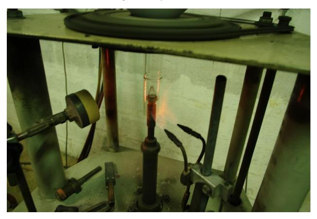
Once the black ring appears around the neck glass, add oxygen to the flame and move in on the button. Positioning of the flame is critical, it should be pointing at the upper edge of the button. If you aim too high, the glass will stretch out too much as it falls, making the joint weak and prone to cracking. Aim too low and the glass won't even touch the button when it falls, then you'll have no choice but to affix a new section of glass and try again.
