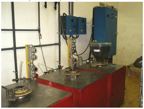
Next lacquer is sprayed for 1 second at low pressure at the tube face, rotating at 90 RPM, running down towards the neck. The tube continues to rotate after spraying for a couple of
