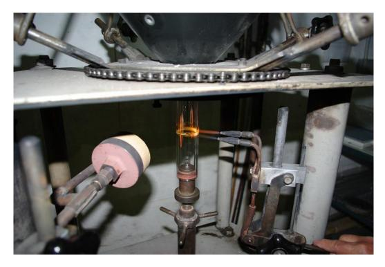
You want the flames to hit both sections of glass equally, so they heat up at the same rate. If the flame heats one section more than the other, the result will be a bad joint because one piece was cooler than the other. After a few seconds the glass will be at the correct temperature, and the lower chuck should be slowly raised so the 2 pieces meet plus an additional 1mm or so to allow the glass to 'mix'.
