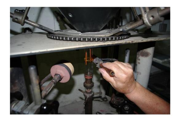
Remove the hydrogen flame, and apply the natural gas burner again. After about 30 seconds, anneal the joint with a medium flame from the natural gas burner. This may be accomplished by reducing the amount of shop air supplied to the burner, or by increasing the supply of natural gas. Anneal the area of the joint for approximately 30 seconds, then bring the burner back to infrared heat.
