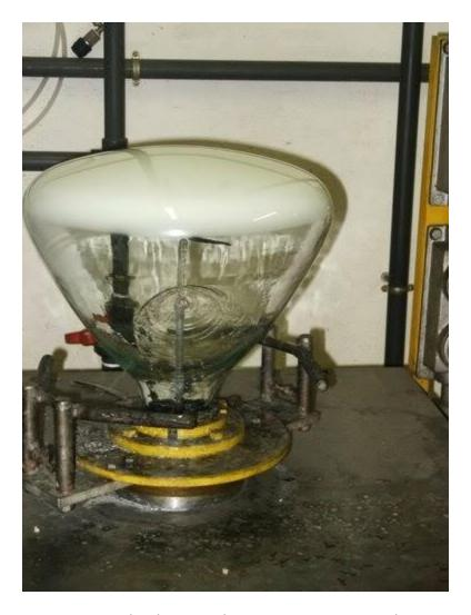
The tube is again sent to the drying rack to remove moisture- there is now a thin coating of lacquer and phosphor, separated by the space formerly occupied by the removed water.
