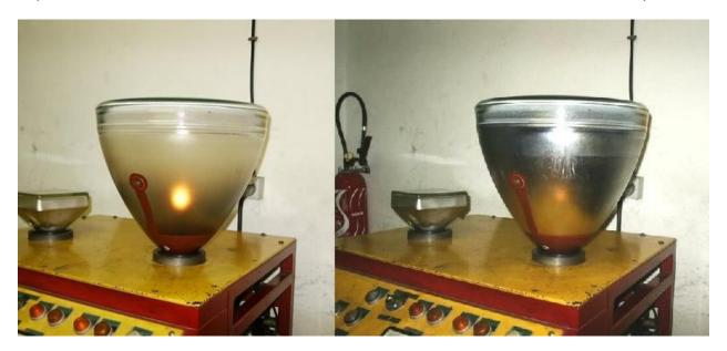
After the coating has been applied, the tube goes into the oven at 410\*C to bake out the remaining lacquer. There is now a thin coating of phosphor and aluminum on the bulb face, separated by the space formerly taken up by the lacquer. A picture tube layer cake! After
