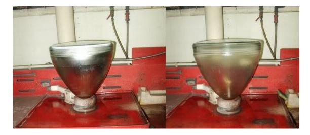
The chemical screening recipe for each tube depends on the size of the bulb and type of phosphor, different mixtures are calculated from the master list for odd sizes. In general the mixture in the tube will contain silicate, phosphor, barium oxide and demineralized water.
