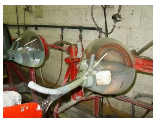
After all the fluid has left the tube, the excess silicate must be 'cut' away from the lower portion of the bulb with a water jet.
