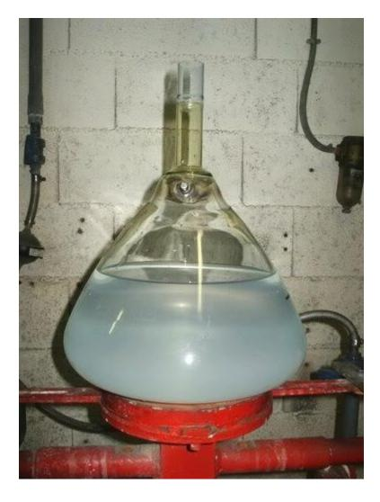
A plastic tube is inserted touching what will be the top of the bulb above the water level, and plastic tape placed onto the neck so that the liquid will not run down the bulb but into the collection trough. The plastic tube lets air into the bulb so that bubbles do not occur as the bulb is slowly tilted, in order for the liquid portion of the mixture to drain off.
