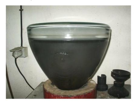
Then it is placed on a heated air drying rack, so the coating can solidify and attach itself properly to the tube face.
