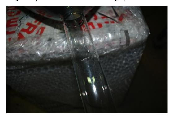
Next position the hot wire around the neck in line with the score in the glass, being mindful that the tips of the tool are to be on either side of the scored line. Turn on the tool, and allow it to heat up. You will hear the glass fracture after about 10-15 seconds, at which point you should remove power from the tool and allow it to cool. The neck should now be fractured all the way around, and you can remove the tool from the neck.
