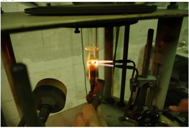
Use the flame to cut the glass off just below the button, and focus the flames at the new joint for a moment to ensure that the glass has fused. Once fused, position the natural gas burner on the new joint for approximately 30 seconds. Anneal with a small blue flame for 20 seconds, then slowly cool the joint by progressively pulling the burner away. Secure all gas, and let the whole thing cool as previously described back to room temperature in the enclosed space.
