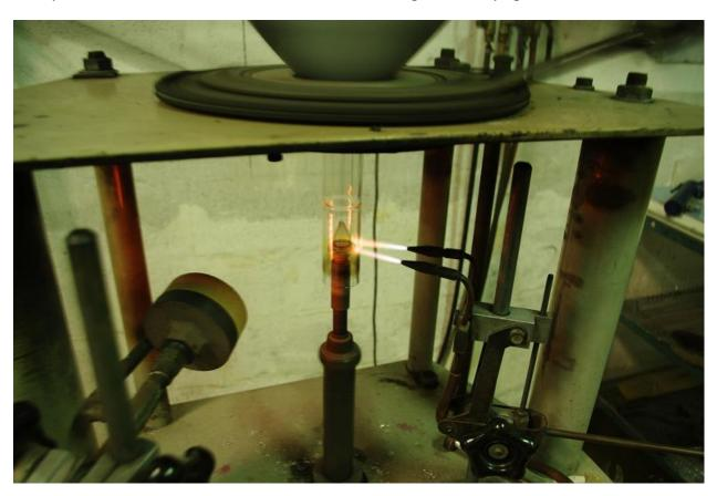
When you notice that the glass has started to melt, follow it on its downward path with the flame. You want to stop it from falling with the graphite paddle, about 1-2" of fall is appropriate.
