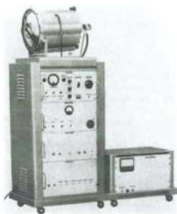
The General Precision Laboratory Model PB-610 projection equipment, with high-voltage supply at right.
