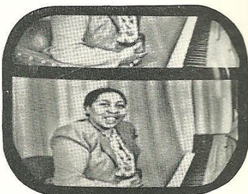
Fig. 91. Vertical free running frequency too low.
