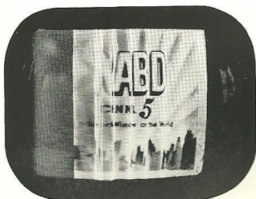
2. Fig. 95. Fold over in the horizontal sweep. Note the horizontal size is reduced considerably.
