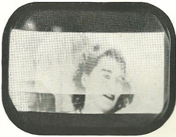
Fig. 90. Vertical free running frequency too high.
