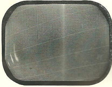
1. Fig. 87. Synchronized raster but no picture.
