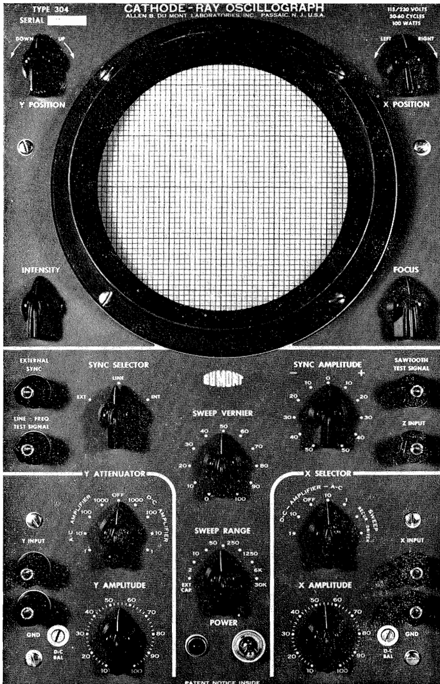
Figure A-2. Front Panel Controls of the Du Mont Model 304 Oscilloscope.
