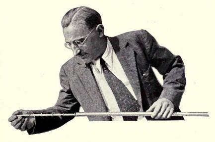
Fig. 45. The Co-axial Cable. The inner conductor has been drawn out of its shield to show how the small insulators are evenly spaced. This shield is made out of flexible aluminum tubing. Dr. C. D. Haigis of Haigis Laboratories, Inc., is demonstrating
