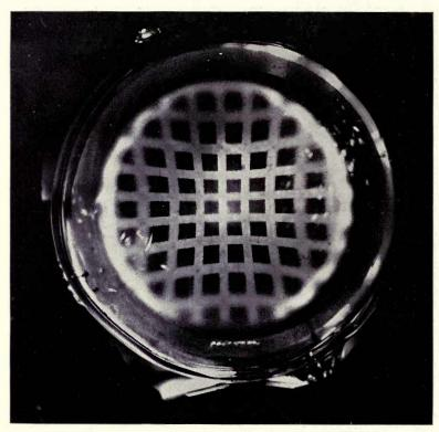
Fig. 76. Image Distortion in Uncorrected Image Tube
