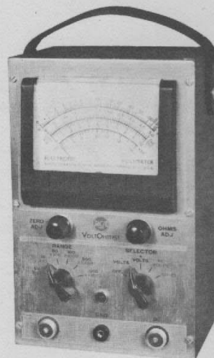
An Electronic Voltmeter and a Test Oscillator are the only Instruments Needed For Alignment
