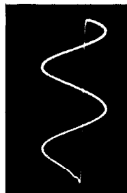
Horizontal (95 Volts PP) Terminal "A" of Sync. Discriminator Transformer (T108)
