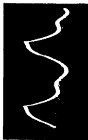
Cathode of Vertical Output (75 Volts PP) (Pin 8 of V122) (6K6GT)
