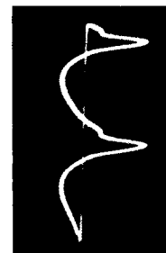
Cathode of Reaction Scanning (60 Volts PP) (Pin 8 of V128) (5V4G)
