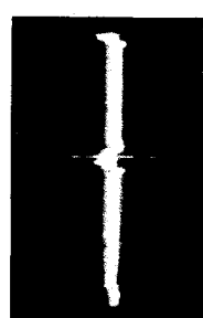
Cathode of Hor. Sync. Discriminator (Pin 5 of V123) (6AL5) Horizontal (.19 Volt PP)
