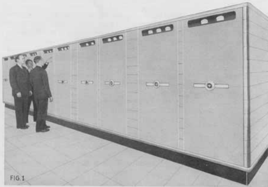
Transmitter for color or fine line television, designed and built by Federal for the Columbia Broadcasting System. It has an output of 1 KW at 500 MC; uniform modulation from DC to 10 MC
