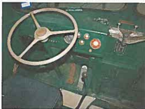
Instrumentation included an air pressure gauge for the air brakes, a tachometer and temperature, fuel and oil pressure gauges.
