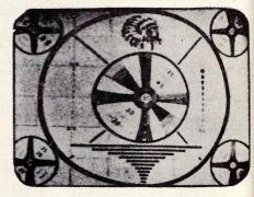
Horizontal linearity out of adjustment
