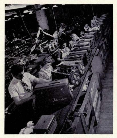
TV CAMERAS BEING ASSEMBLED Courtesy RCA
