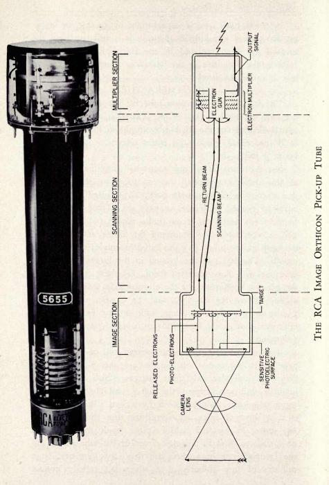
silver oxide. The back of the mica is coated with colloidal graphite, a conductor which is directly connected to the output of the tube externally.
