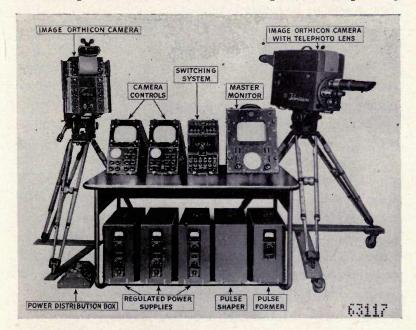
NECESSARY BASIC STATION EQUIPMENT FOR REMOTE PICK-UPS
