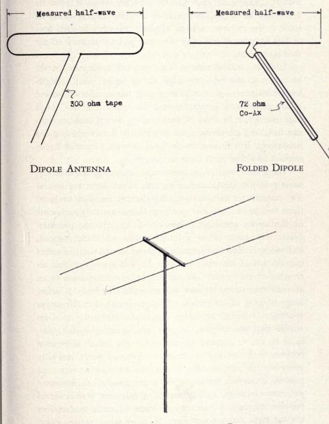
DIPOLE RECEIVING ANTENNA WITH REFLECTOR
