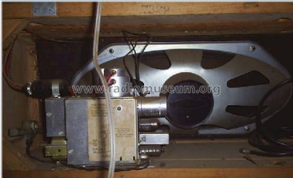
Remote Control Chassis Assembly as installed in General Electric Television circa 1959. TV Chassis M5 & U4 model numbers include: 21C3559, 21C3567, 21C3570, 21C3571, 21C3573, 21C3575, 21C3576, 21C3580, 21C3581, 21C3585, 21C3586 and others?
