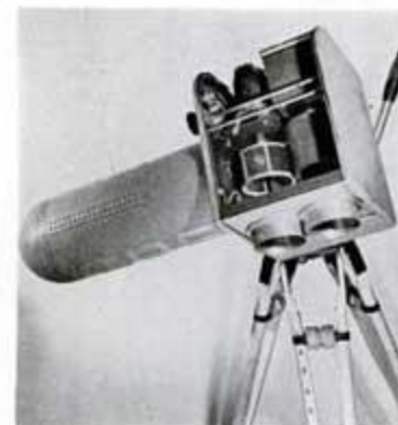
COLOR TELEVISION CAMERA mounts the camera tube on its side. Lenses point down. Above left lens is the color drum.
