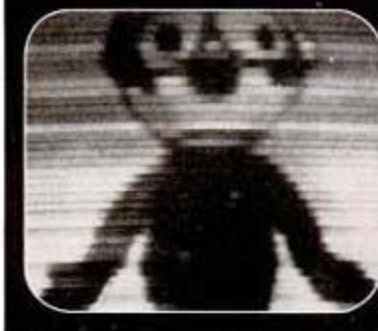
1929 picture was produced by a mechanical, not an electronic, scanning. With only 80 lines very little detail comes through.
