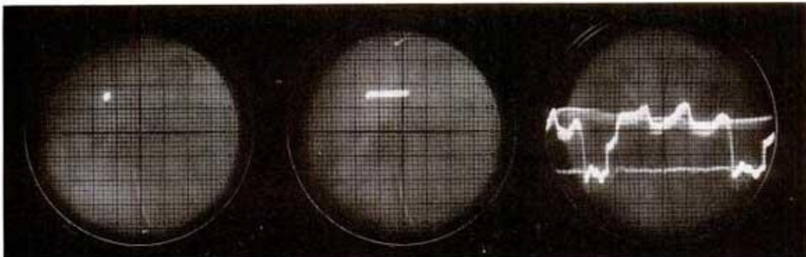
POINT OF LIGHT glows on tube face as beam is held still. This is laboratory oscilloscope tube, cousin of the television tube.
