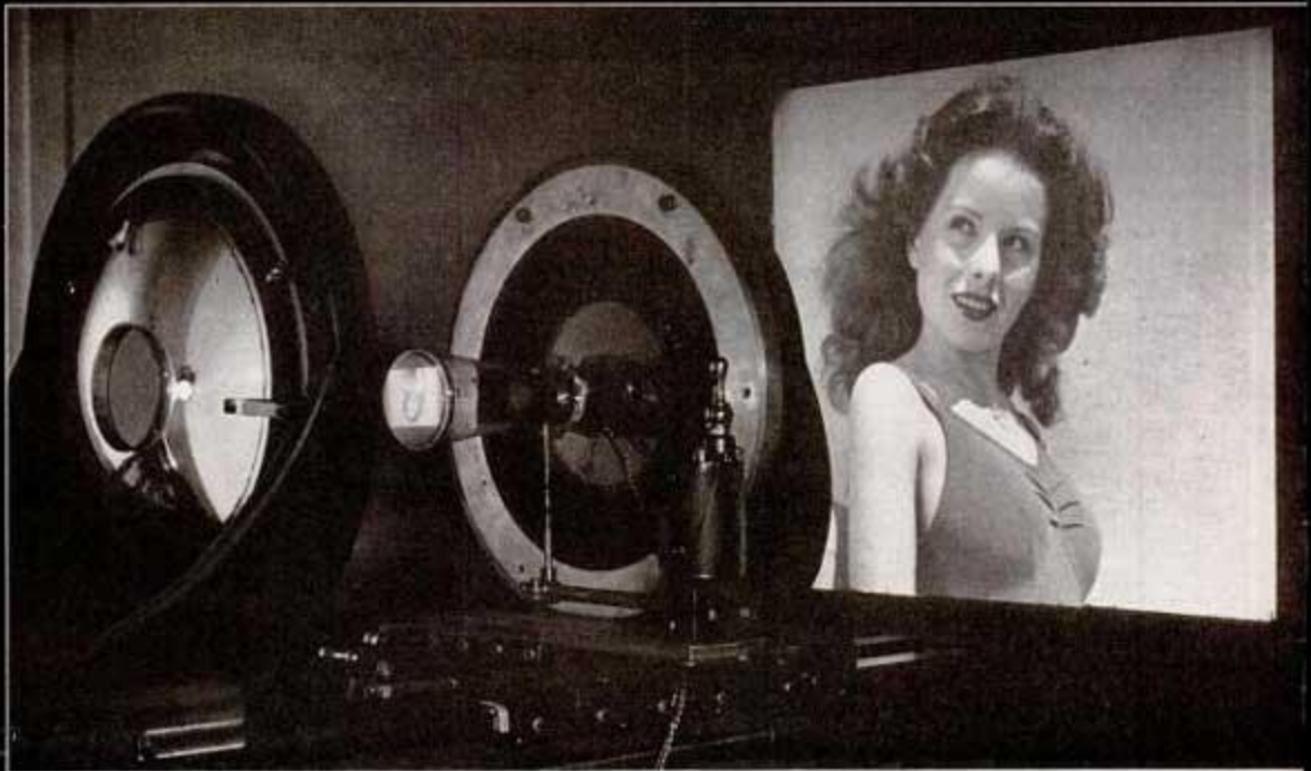
SCHMIDT PROJECTION system is an adaptation of Schmidt reflecting telescope. Image on small, 4-inch television tube (center) is pointed at the spherical mirror at left. The mirror reflects and projects image back through large lens in which tube is mounted and onto big screen. The tube would block light reflected from center of mirror—hence hole in the mirror.
