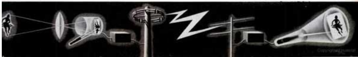
TELEVISION SEQUENCE: IMAGE FOCUSED ON PLATE, SCANNED BY BEAM (SEE TOP) IS TRANSLATED INTO RADIO SIGNAL, BROADCAST, TRANSLATED BACK INTO IMAGE BY RECEIVING SET
