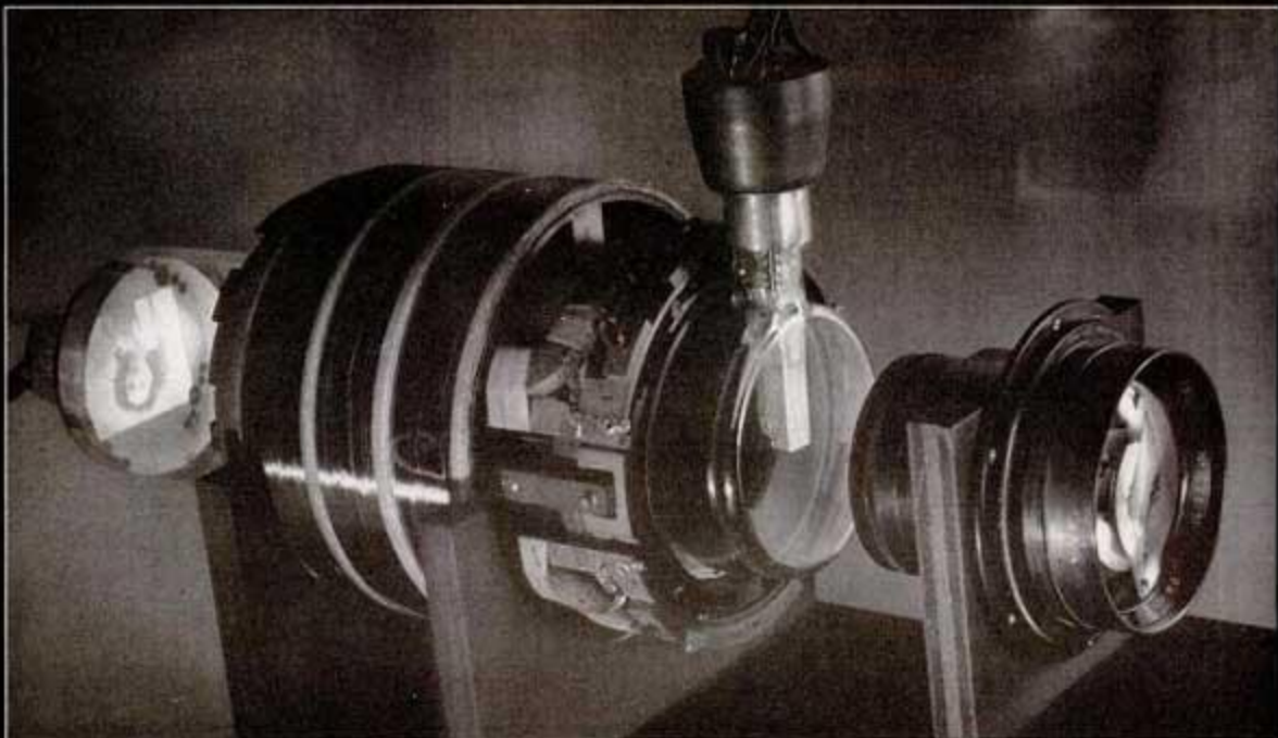
DISSECTOR CAMERA TUBE was developed by Fernseh Television and Radio Corp. Image is focused on light-sensitive plate (left). Electrical field transfers visible image into extended electronic image (top, opposite page). Electromagnetic field pulls this extended image back and forth in front of scanning finger mounted vertically at front of the tube.
