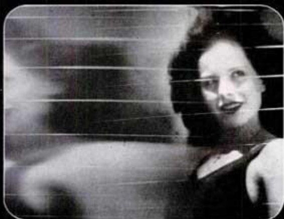
GHOST IMAGE at the left is drawn by horizontal return trace of beam as it sweeps back across the screen from right to left. Ghost image is blanked out in television reception.
