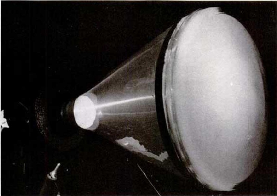
PICTURE TUBE reverses operation performed by camera tube shown on preceding page. It translates radio signal into visi-
