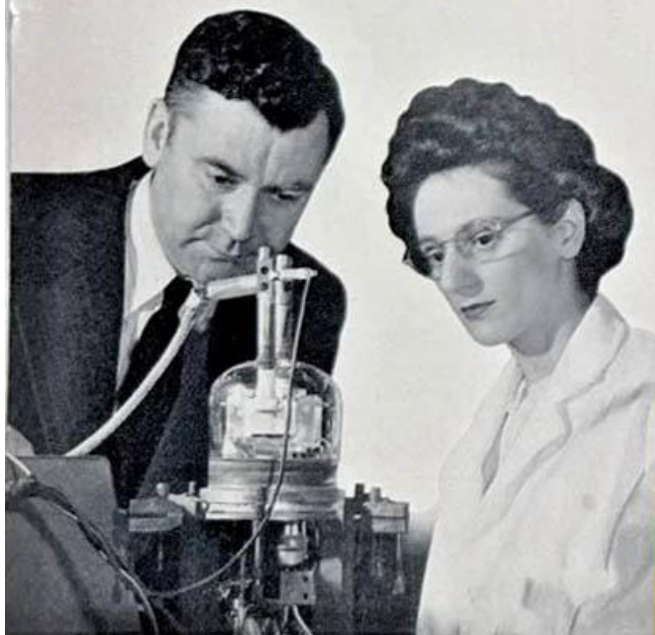
The RCA 5-kilowatt television transmitter tube is water-cooled through a system of silver-plated copper channels.
