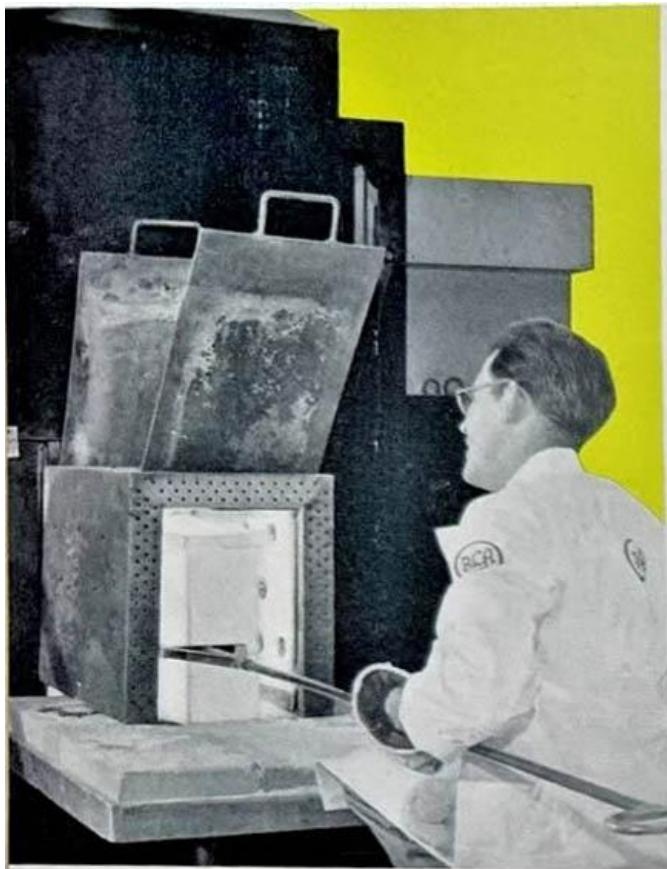
After this white-hot block of luminescent material is removed from the furnace, it will be spread on the face of a kinescope to serve as a "screen" on which television pictures will appear.
