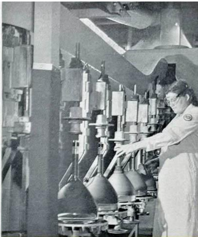
As television picture tubes near the end of the production line, they are sprayed with an outer coating of graphite paint, the final process before shipment.
