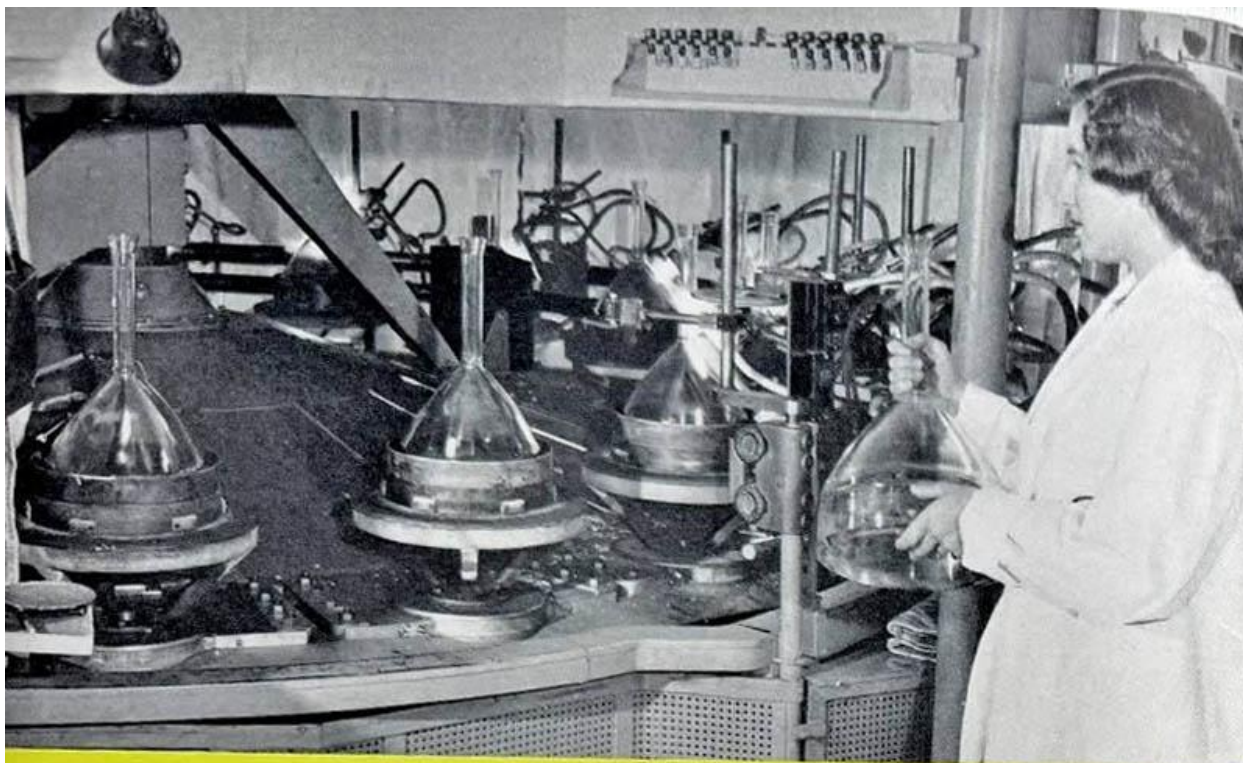
While torch-like fingers of flame shoot out automatically to play upon the glass bulbs, radio-heat is applied to speed the production of television's electronic picture tubes.
