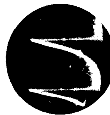
INPUT OF SYNC. AMPL. PIN 4, V16A 'SCOPE AT 7875 C.P.S. 26V. P-P
