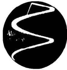
LUG No. 1 HORIZ. OUTPUT TRANSFORMER SCOPE AT 7875 C.P.S. 46V. P-P
