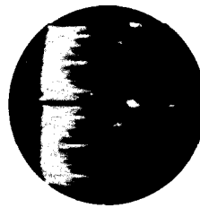
INPUT, 1st VIDEO AMPL. PIN 2, V14A 'SCOPE AT 30 C.P.S. 3V. P-P
