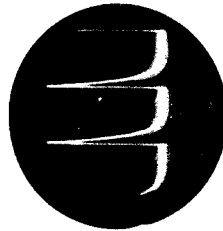
OUTPUT, SYNC CLIPPER PIN 3, V17B 'SCOPE AT 5250 C.P.S. 15V. P-P
