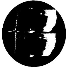
OUTPUT OF SYNC CLIPPER PIN 1, V17B 'SCOPE AT 30 C.P.S. 80V. P-P
