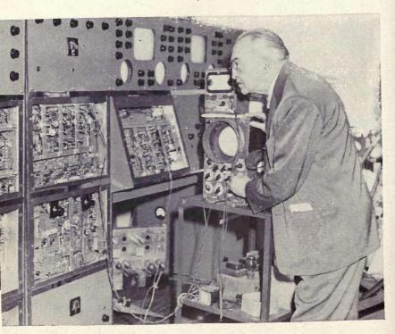
Here the author uses an oscilloscope for testing a circuit. The "lazy Joe" patterns which appear indicate to television experts where in the "bird's nest" the trouble is.
