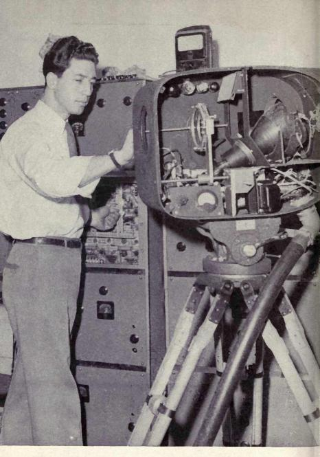
We see here a television camera with the side removed so that we can learn a little about the maze of wires and strange tubes and lenses which make up its working parts. The large conduit leading from the front of the camera is a coaxial cable.
