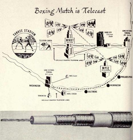
The coaxial cables carry television broadcasts over areas where relay stations are not feasible. Pictured are peeled-back sections of three types of coaxial cables.
