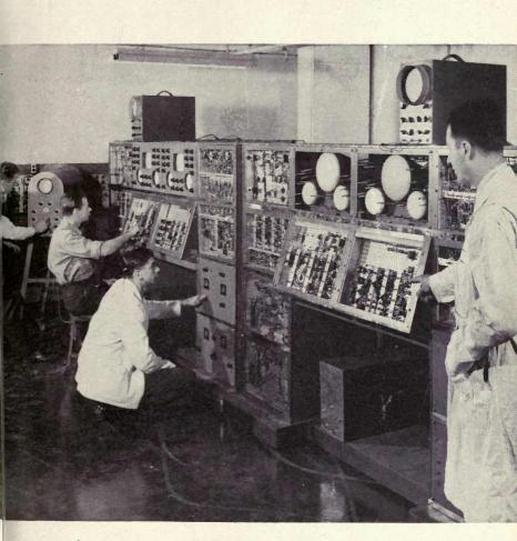
The control room is a busy place, but no one rushes about. Each control operator must watch the screens to which he is assigned, and instantly select the scene which is best suited to be broadcast. A flick of a switch changes the broadcast from one screen to another.
