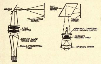
A simple projection system using a Application of the Schmidt system magnifying lens unit.
