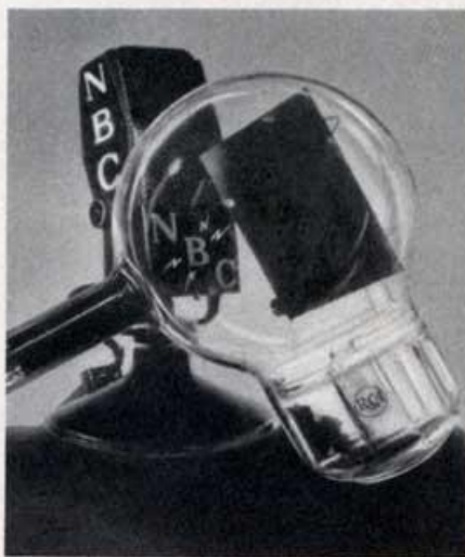
The television eye, RCA's Iconoscope, looking much like a glass bubble with a sheet of metal inside, is the device which transforms what it sees into electrical impulses. The ear of television is the microphone which picks up the sound and gives voice to the receiver.
