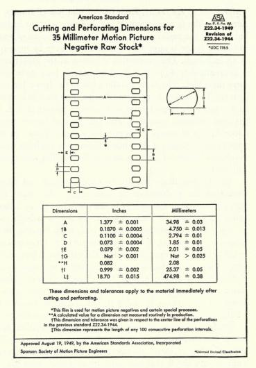
Fig. 1-1. Dimensions and details of 35 mm film stock showing perforations and general appearance. Frame size (camera) 0.868 by 0.631 inches. Projector aperture is 0.825 by 0.600 inches.
