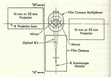
Fig. 4-10. Floor layout for two projectors operating with multiplexer.
