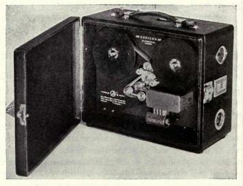
Fig. 3-14. Auricon sound recorder for portable work is very similar to a simple camera in mechanical details. With this recorder and synchronized camera full lip sync films can be made. Or it can be used for double system with the Auricon Pro camera.
