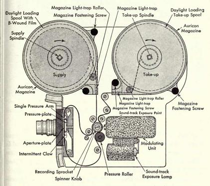
Fig. 3-5. Diagram of film path through the Auricon camera. It is clear how, by the time the film reaches the sound recorder, all intermittent movement has been smoothed out. This type of camera provides extreme economy in operation.
