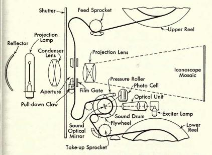
Fig. 4-17. Diagram of film path and mechanism of the RCA 16 mm projector.
