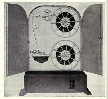
Fig. 3-19. Neumade film cleaner for 16 mm film.
