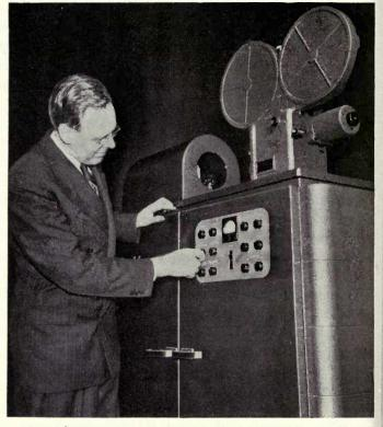
Fig. 5-2. RCA film recording equipment. A high voltage projection type cathode-ray tube is housed on the left-hand top cover, a film camera—either 16 mm or 35 mm—is on the right, and below are the controls and auxiliary equipment.
