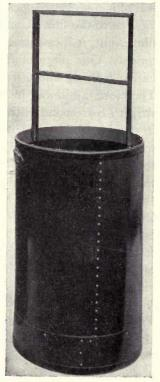
Fig. 9-2. Neumade editing rack and barrel.
