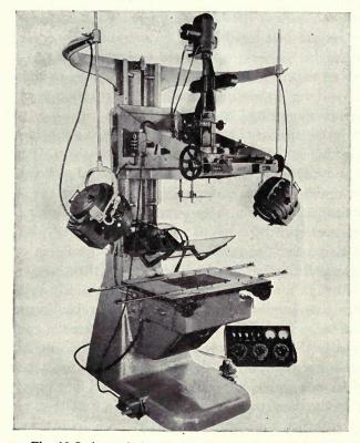
Fig. 10-5. Acme Animation Stand. Any lighting effect desired is possible with the table and lights shown. One to three films can be run through the camera at the same time. A foot control operates the camera leaving the operator's hands free. Zooms are possible of course, and the camera can be moved to follow any line or path desired. All types of effect can be made, including dissolves. Compressed air is used to move the camera and platen. CHAPTER 11
