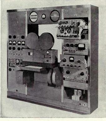
Fig. 3-16. This view of the new RCA unit construction film recording rack at Chicago shows how each of the individual chasses are mounted on pivots in pull-out slide tracks to facilitate servicing. Each chassis can be pulled out like a drawer to provide easy access to elements on the upper side and may then be tilted, as shown in this photo, to expose circuit connections and components on the underside.
