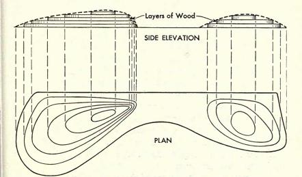
Fig. 20-1. Miniature construction showing layers of wood, and foundation to be covered with plaster laid over chicken wire or papier maché laid over wood.
