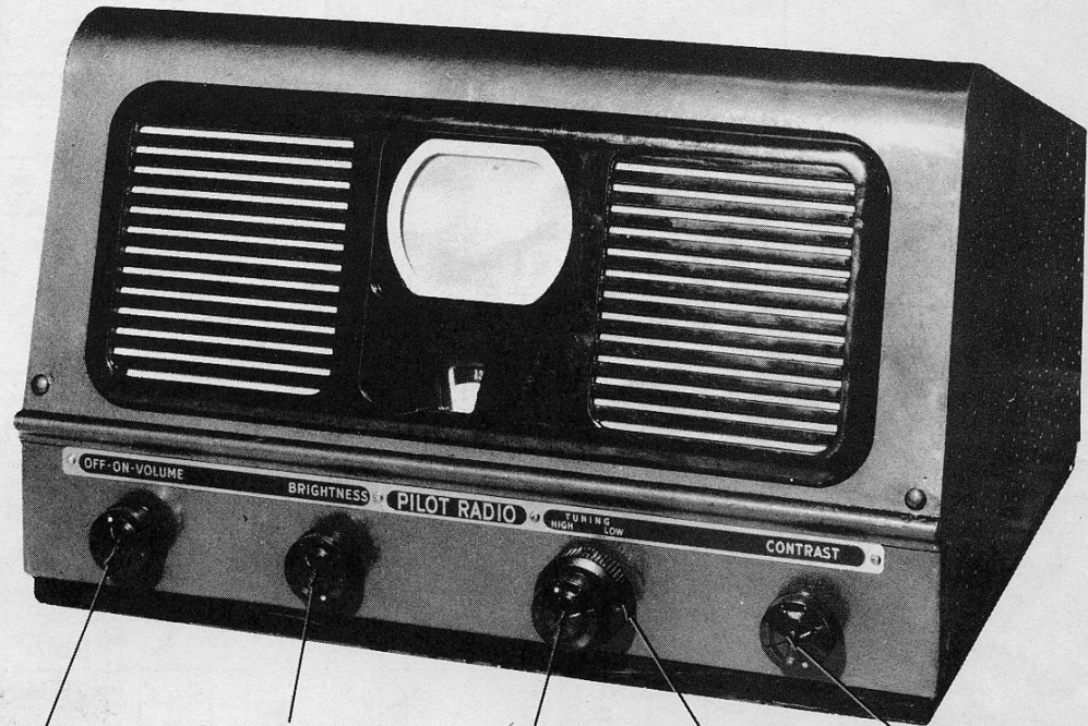
VOLUME CONTROL ON-OFF SWITCH BRIGHTNESS CONTROL HI-LO BAND SWITCH TUNING CONTROL CONTRAST CONTROL
