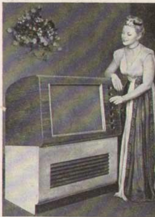
This is a CBS color-television receiver. It uses a projection system to fill its giant 21-inch screen
